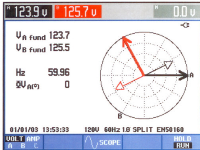
Phasor diagram (Voltage) of ER Water Torch in operation, note phase angle difference
